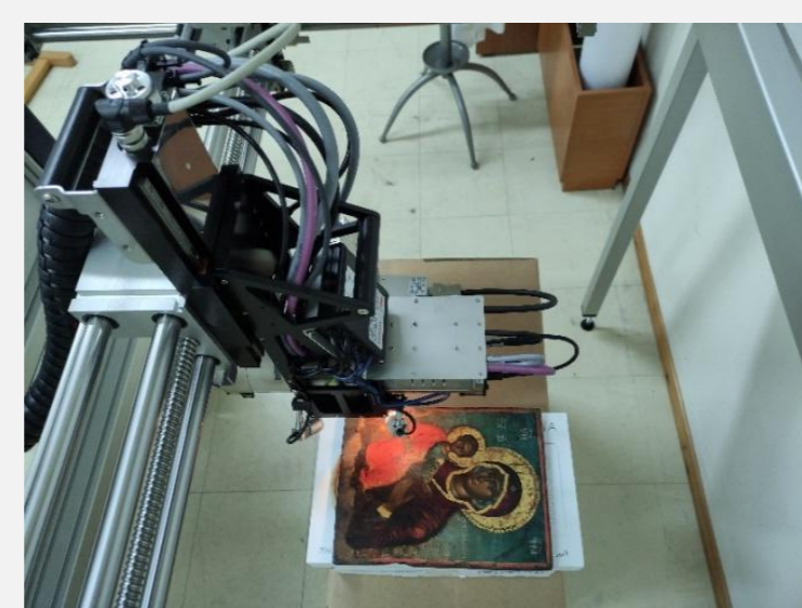
Figure 1: M6 Jetstream (Bruker) MA-XRF Scanner.
