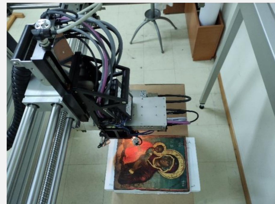
Figure 1: M6 Jetstream (Bruker) MA-XRF Scanner.
